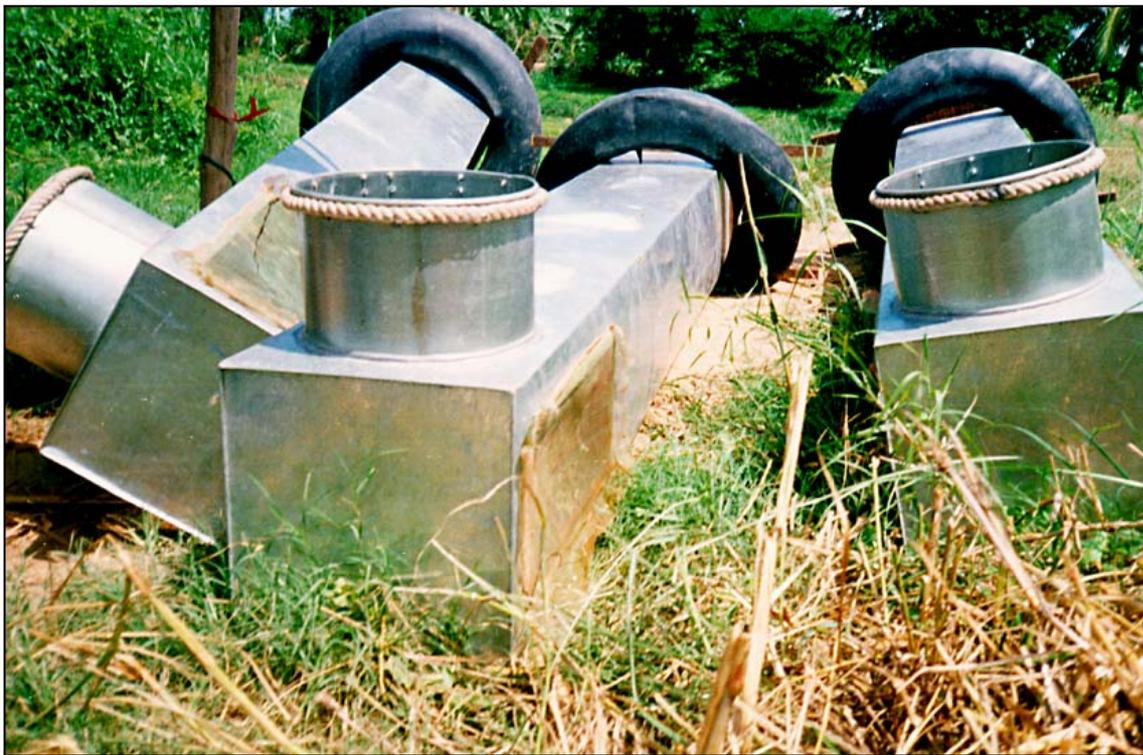
Figure 36: The water current entering the capture room splits into three currents: two lateral ones, escaping through the mosquito netting and a third current, that transports the fry to the water surface, where it is scooped out.
